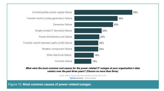
Data center managers will not be surprised that failure of uninterruptible power supplies (UPSs), transfer switches and generators (usually failing to start) cause most power-related outages. These devices are a last line of defense, often for very large numbers of servers and IT equipment.
